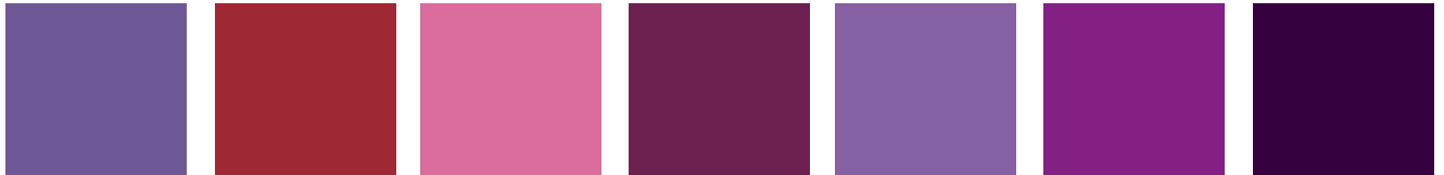
RAL 4001 HBW 18 ● RAL 4002 HBW 12 ● RAL 4003 HBW 25 ● RAL 4004 HBW 7 ● RAL 4005 HBW 20 ● RAL 4006 HBW 13 ● RAL 4007 HBW 6 ● RED PURPLE ● RED VIOLET ● ERICAVIOLET ● BORDEAUX VIOLET ● BLUE PURPLE ● TRAFFIC PURPLE ● PURPLE VIOLET ●
