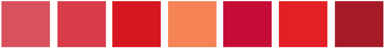
RAL 3017 HBW 22 ● RAL 3018 HBW 19 ● RAL 3020 HBW 14 ● RAL 3022 HBW 26 ● RAL 3027 HBW 13 ● RAL 3028 HBW 17 ● RAL 3031 HBW 14 ● ROSÉ ● STRAWBERRY RED ● TRAFFIC RED ● SALMON RED ● RASPBERRY RED ● PURE RED ● ORIENT RED ●
